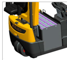
Sideway battery box
