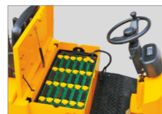
Large capacity batteries located in the lowest part of frame, offers low centre of gravity.
