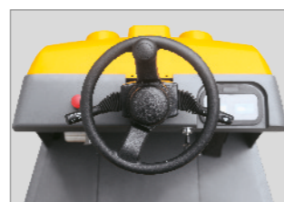
Adjustable steering column with electric F/R lever.
